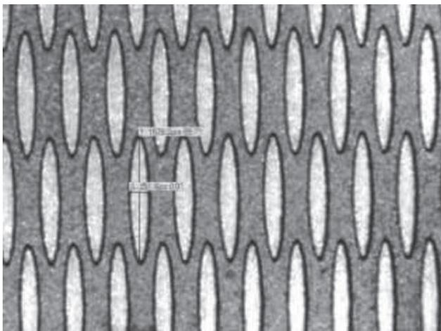
**Fig. 4** An experimental screen-printed sharkskin surface designed by U. Leeds. (Image courtesy of N. Kapur)
