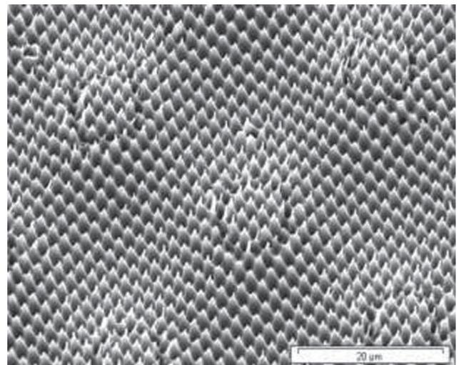
Fig. 2 Artificial Lotus effect surface created by MacDermid Autotype. (Image courtesy of Creavis)
